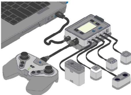
Plug all devices into the Robot Brain, and plug the Robot Brain into your computer via USB.
