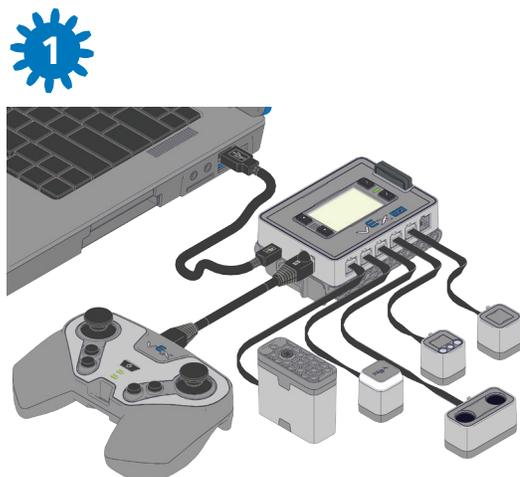
Plug all devices into the Robot Brain, and plug the Robot Brain into your computer via USB.
